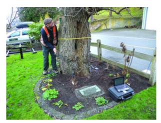
Scott Baker, a consulting arborist with Seattle-based Tree Solutions Inc., taps sensors of a tomograph into the Fowler Pear Tree in Old Town. The device uses sound waves to produce 3-D images that help arborists analyze the overall health of the tree.
